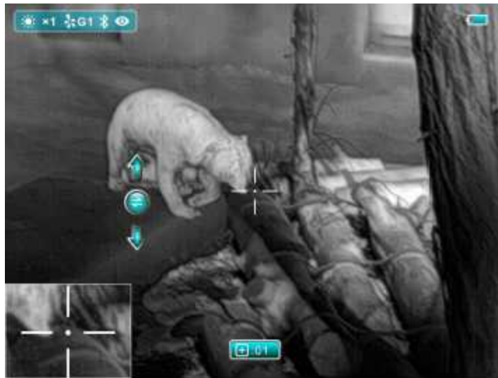
Figure5 Blind pixel calibrating function
