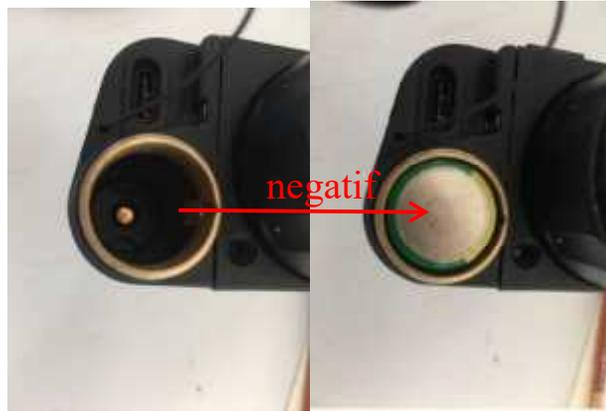
Fig. 7-1 Schematic diagram of battery installation
